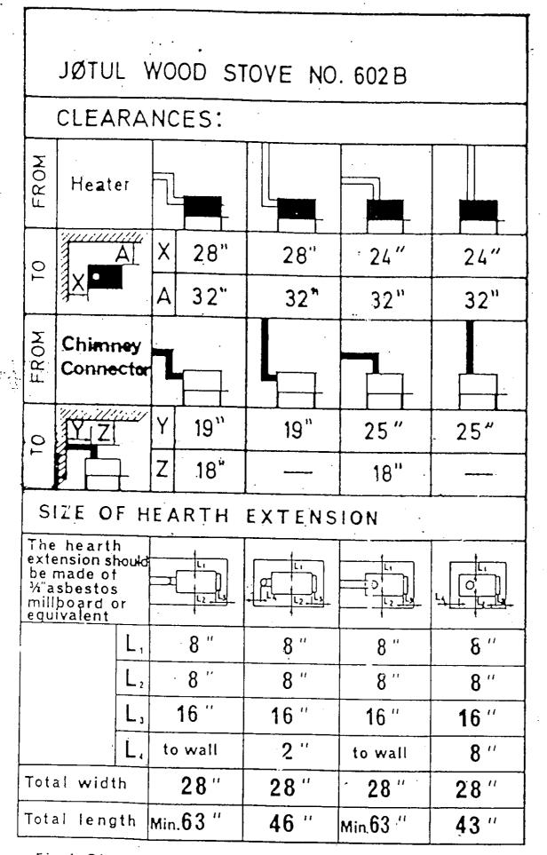
Fig.1 Clearances and Hearth Extension Size
